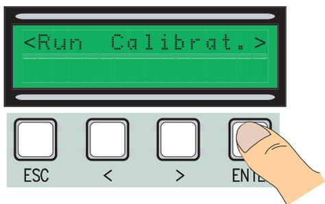
**[2]** Perform a complete opening run using (< >) until reaching the maximum opening point
