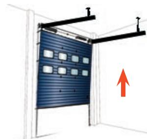
**[4]** Perform a full closing run by using (< >), until reaching the maximum closing point
