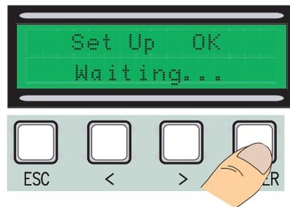
**[12]** If the calibration has not been performed correctly, the "reprogram" message will appear and you will return to step 1.
